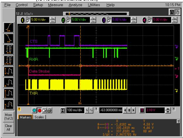
FIGURE 2-13: HOST CONTROLLER RECEPTION (P  $\rightarrow$  S) OF A 250 BYTE PACKET (FROM PIC IRDA STANDARD STACK)
