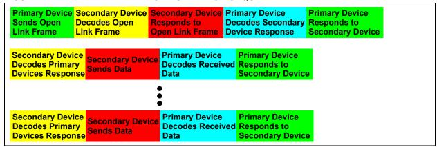
FIGURE 2-12: HOST CONTROLLER TRANSMISSION (S  $\rightarrow$  P) OF A 250 BYTE PACKET (TO PIC IrDA STANDARD STACK)
