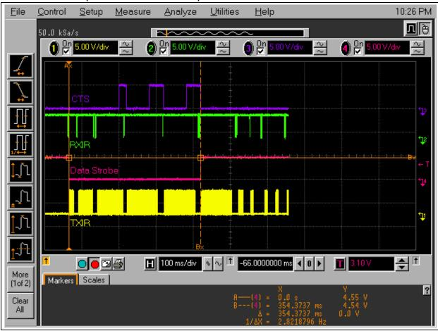
FIGURE 2-15: HOST CONTROLLER TRANSMISSION (S  $\rightarrow$  P) OF A 250 BYTE PACKET (TO PDA HP IPAQ H2495B)
