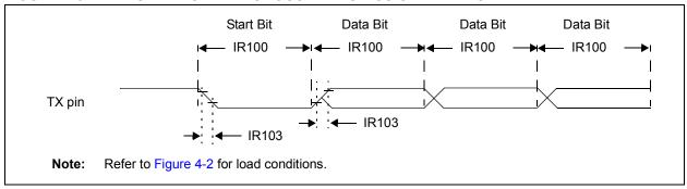
TABLE 4-5: UART ASYNCHRONOUS TRANSMISSION REQUIREMENTS
