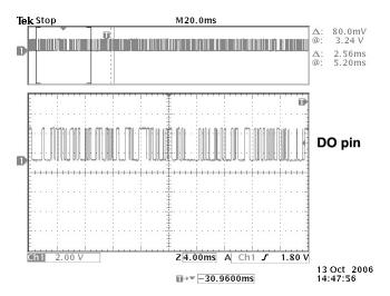
Figure 8. Data Out Pin with No Squelch (SQ = 1).
