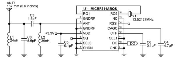
433.92 MHz, 1kHz Baud Rate Example
