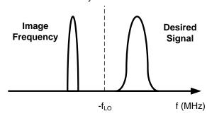
Figure 6. Low Side Injection Local Oscillator.
