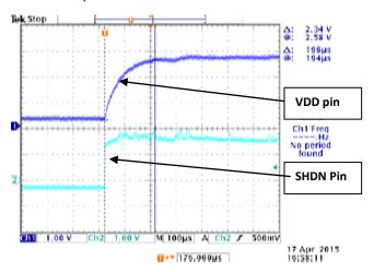
The suggestion provided above will generally serve to prevent the startup issue from happening to the MICRF211 series ASK receiver. However, exact values of the RC network depend on the ramp rate of the supply voltage, and should be determined on a case-by-case basis.
