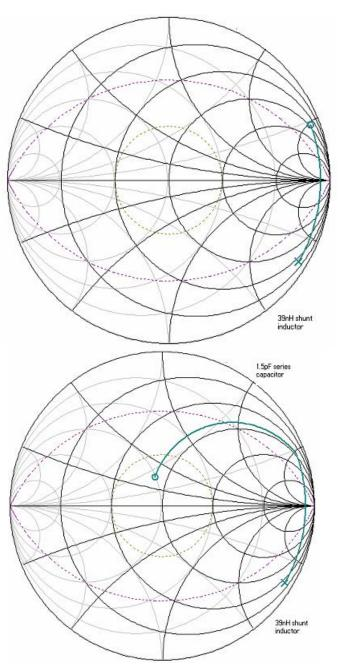
Figure 5. Plotting the Shunt Inductor and Series Capacitor.
