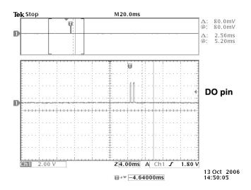
Figure 9. Data Out Pin with Squelch (SQ = 0).
