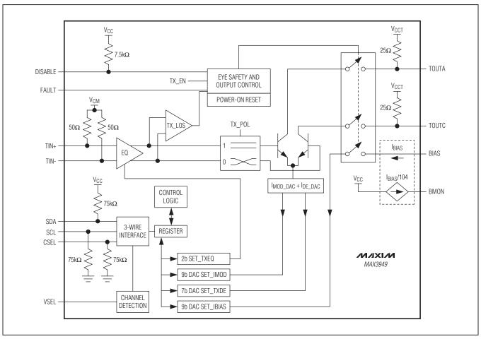
Figure 2. Functional Diagram
