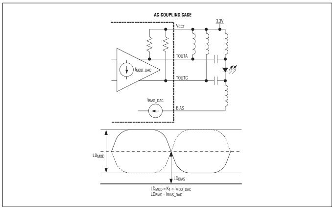
Figure 3. AC-Coupling Case
