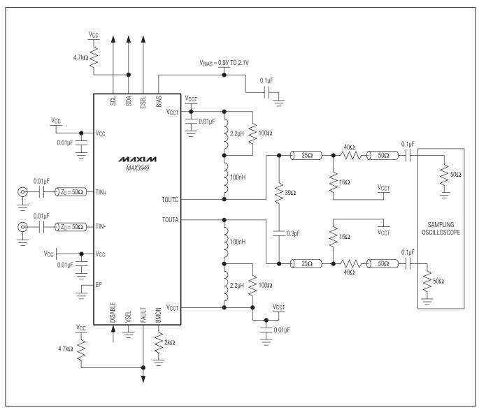
Figure 1. AC Test Setup
