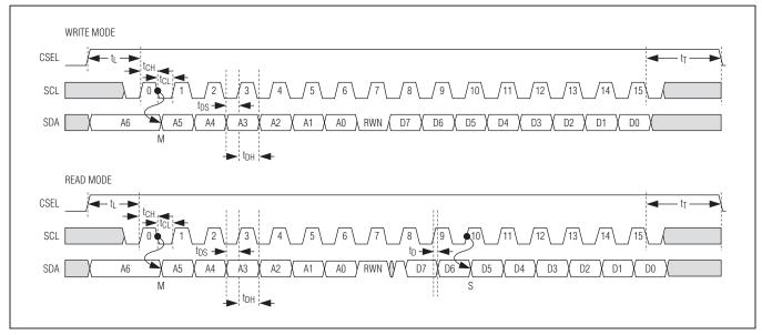
Figure 5. Timing for 3-Wire Digital Interface
