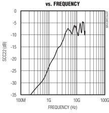
INPUT DIFFERENTIAL TO COMMON-MODE **RETURN LOSS vs. FREQUENCY**
