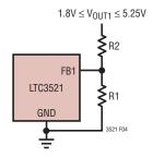
Figure 4. Setting the Buck-Boost Output Voltage
