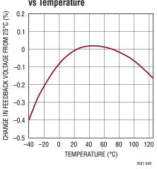
**Buck Feedback Voltage** vs Temperature
