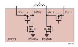
Figure 1. Buck-Boost Switch Topology
