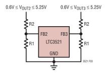
Figure 3. Setting the Buck Output Voltage
