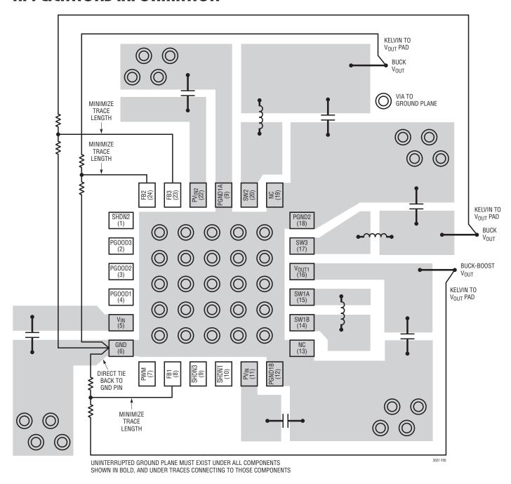
Figure 5. LTC3521 Recommended PCB Layout
