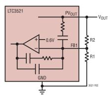
Figure 2. Buck-Boost Error Amplifier and Compensation
