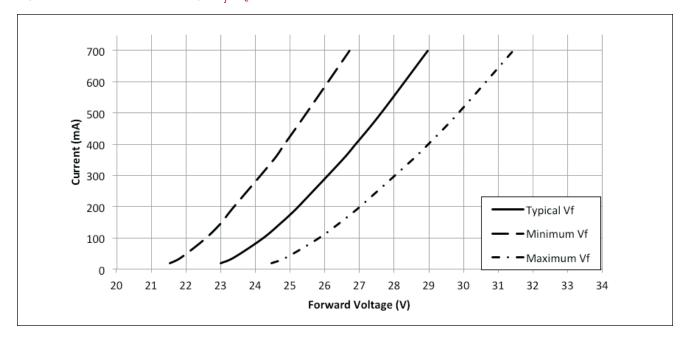
Figure 2: Drive Current vs. Voltage ( $T_i = T_c = 25^{\circ}C$ )
