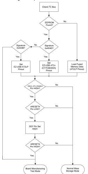
Figure 9. Operational Mode Selection Flow
