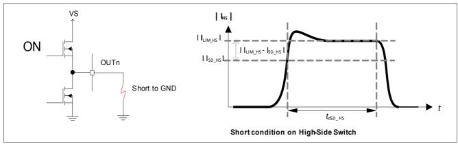
Figure 6 High-Side Switch - Short Circuit and Overcurrent Protection
