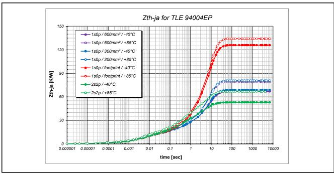
Figure 16 ZthJA Curve for different PCB setups
