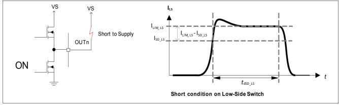
Figure 7 Low-Side Switch - Short Circuit and Overcurrent Protection
