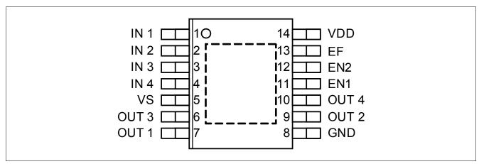
Figure 1 Pin Configuration TLE94004EP with direct interface
