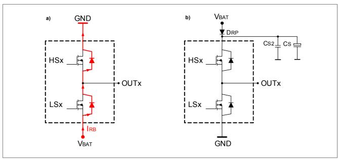
Figure 4 Reverse Polarity Protection
