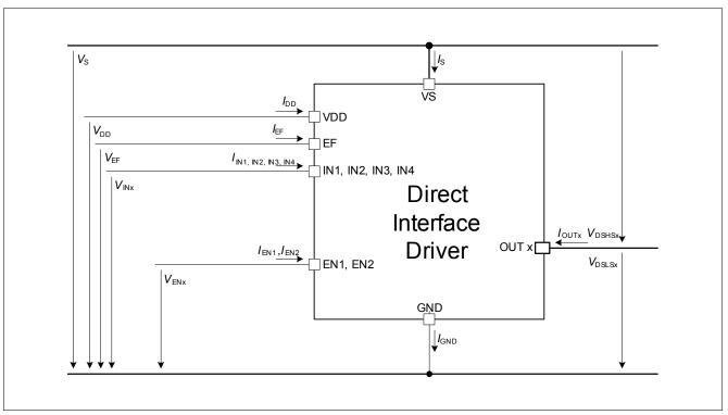
Figure 3 Voltage and Current Definition
