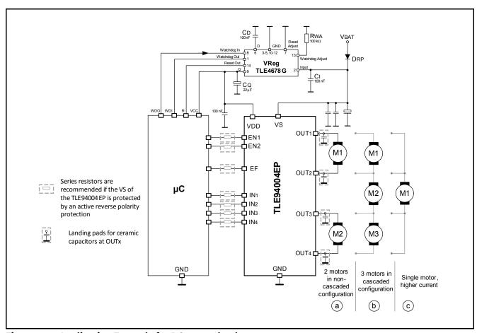
Figure 13 Application Example for DC-motor loads
