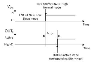
Figure 5 Output setup time after a transition from standby to normal mode
