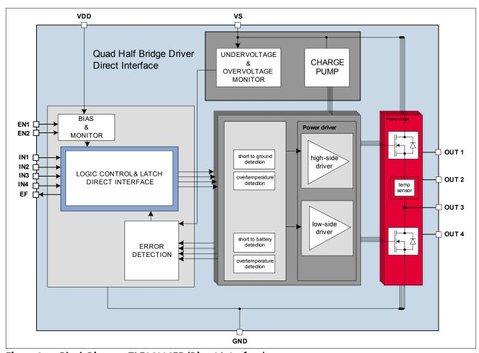
Figure 2 Block Diagram TLE94004EP (Direct Interface)
