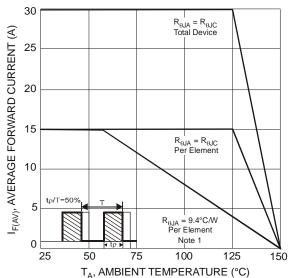
Fig. 5 Forward Current Derating Curve
