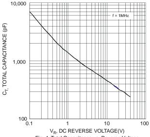
Fig. 4 Total Capacitance vs. Reverse Voltage
