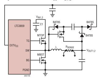
Figure 9. Capacitive Charge Pump for EXTV<sub>CC</sub>
