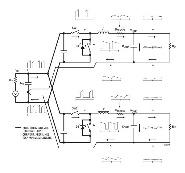
Figure 11. Branch Current Waveforms for Bucks
