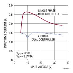
Figure 2. RMS Input Current Comparison
