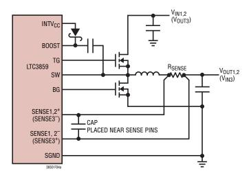
4a. Using a Resistor to Sense Current
