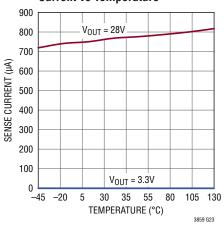
Boost SENSE Pin Total Input Current vs Temperature
