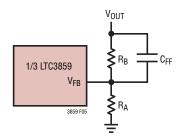
Figure 5. Setting Output Voltage
