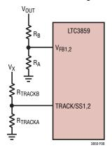
Figure 8. Using the TRACK/SS Pin for Tracking
