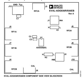
Figure 2. ADG936x Evaluation Board Top View
