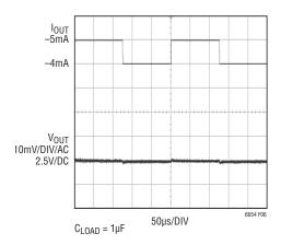
Figure 6. LT6654-2.5 Sinking 4mA to 5mA
