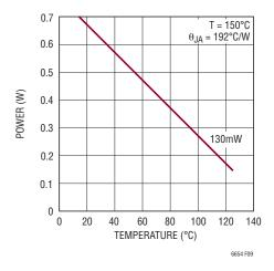
Figure 9. Maximum Allowed Power Dissipation of the LT6654
