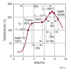
Figure 12. Lead Free Reflow Profile
