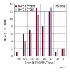
Figure 13. Output Voltage Shift Due to IR Reflow (%)
