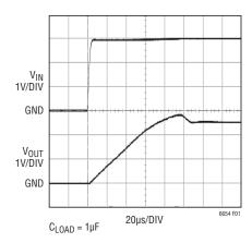
Figure 1. Turn-On Characteristics of LT6654-2.5
