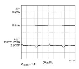
Figure 4. LT6654-2.5 Sourcing and Sinking 0.5mA
