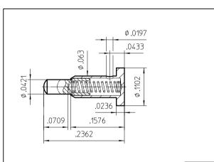
Note: Contact P/N is for basic contact, please add suffix for plating code and, for socket contacts, assembly code.
