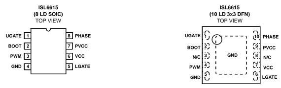
RECOMMEND TO CONNECT PIN 3 TO GND AND PIN 8 TO PVCC
