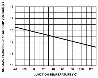
FIGURE 12. AHB - AHS, BHB - BHS NO-LOAD CHARGE PUMP VOLTAGE vs TEMPERATURE
