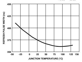
FIGURE 16.  $tT_{REF-PW}$  REFRESH PULSE WIDTH vs TEMPERATURE
