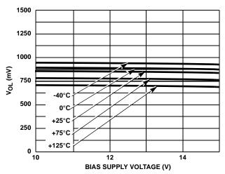
FIGURE 26. LOW LEVEL OUTPUT VOLTAGE  $V_{OL}$  vs BIAS SUPPLY AND TEMPERATURE AT  $100\mu\text{A}$
