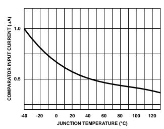
FIGURE 9. COMPARATOR INPUT CURRENT I<sub>L</sub> vs TEMPERATURE AT  $V_{CM} = 5V$
