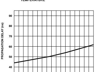
FIGURE 18. UPPER TURN-OFF PROPAGATION DELAY  $t_{\mbox{\scriptsize HPHL}}$  vs TEMPERATURE
