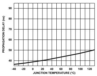
FIGURE 20. LOWER TURN-OFF PROPAGATION DELAY  $t_{\mbox{\scriptsize LPHL}}$  vs TEMPERATURE
