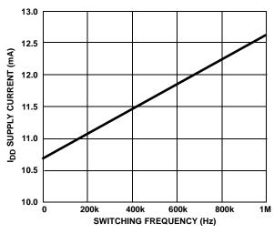
FIGURE 5. I<sub>DDO</sub> NO-LOAD I<sub>DD</sub> SUPPLY CURRENT vs FREQUENCY (Hz)
