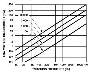
FIGURE 29. LOW VOLTAGE BIAS CURRENT I<sub>DD</sub> AND I<sub>CC</sub>
