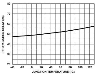
FIGURE 17. DISABLE TO LOWER ENABLE  $t_{\text{DLPLH}}$  PROPAGATION DELAY vs TEMPERATURE
