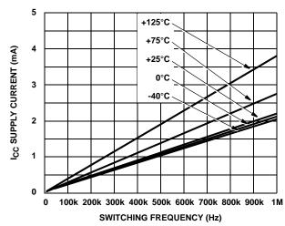
FIGURE 7. I<sub>CCO</sub>, NO-LOAD I<sub>CC</sub> SUPPLY CURRENT vs FREQUENCY (Hz) TEMPERATURE
