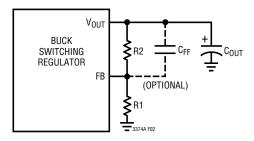
Figure 2. Feedback Components
