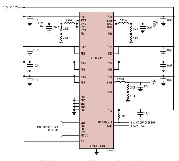
Figure 5. Combined Buck Regulators with Common Input Supply (4A, 3A, 1A)
