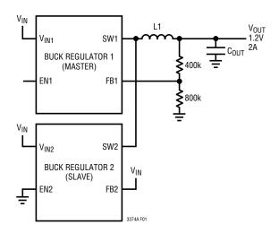
Figure 1. Buck Regulators Configured as Master-Slave
