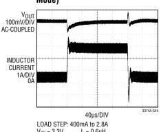
LOAD STEP: 400mA to 2.8A  $V_{IN}$  = 3.3V L = 0.6 $\mu$ H  $V_{OUT}$  = 1.8V
