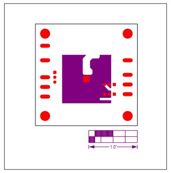
Figure 18. MAX17544 5V Output EV Kit Component Placement Guide—Bottom Solder Mask
