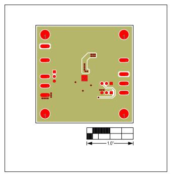
Figure 16. MAX17544 5V Output EV Kit PCB Layout—Solder Side
