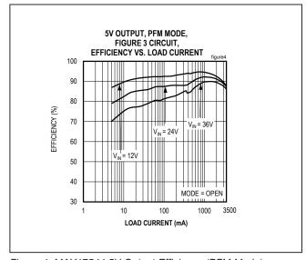
Figure 4. MAX17544 5V Output Efficiency (PFM Mode)
