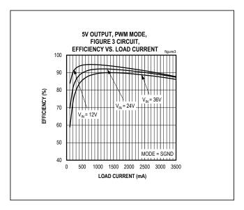
Figure 3. MAX17544 5V Output Efficiency (PWM Mode)
