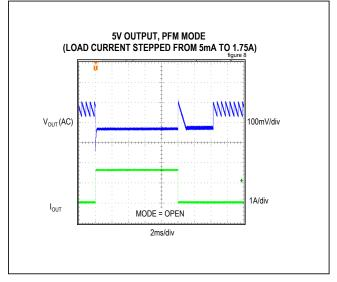
Figure 8. MAX17544 5V Output, 5mA to 1.75A Load Transient (PFM Mode)
