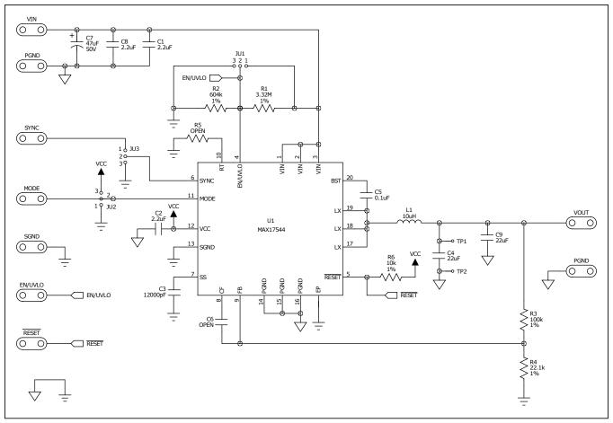
Figure 11. MAX17544 5V Output EV Kit Schematic
