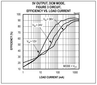
Figure 5. MAX17545 5V Output Efficiency (DCM Mode)
