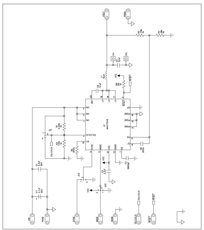
Figure 11. MAX17545 5V Output EV Kit Schematic
