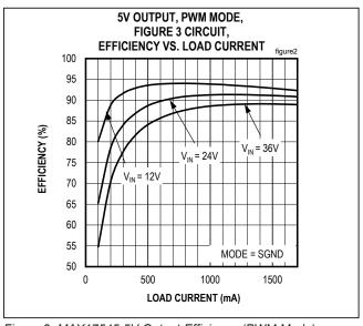
Figure 2. MAX17545 5V Output Efficiency (PWM Mode)
