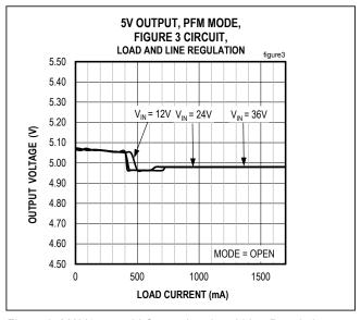
Figure 3. MAX17545 5V Output Load and Line Regulation (PFM Mode)
