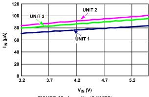
FIGURE 42.  $I_{IN}$  vs  $V_{IN}$  (3 UNITS)
