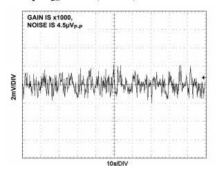
FIGURE 26.  $V_{OUT}$  NOISE, 0.1Hz TO 10Hz
