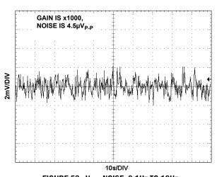
FIGURE 53.  $V_{OUT}$  NOISE, 0.1Hz TO 10Hz
