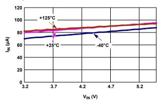
FIGURE 43.  $I_{\rm IN}$  vs  $V_{\rm IN}$  over temperature
