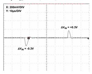
FIGURE 9. LINE TRANSIENT RESPONSE, NO CAPACITIVE LOAD
