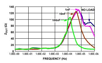
FIGURE 12.  $Z_{OUT}$  vs FREQUENCY
