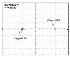
FIGURE 22. LINE TRANSIENT RESPONSE, NO CAPACITIVE LOAD
