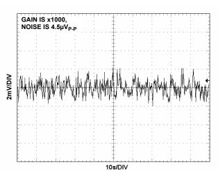
FIGURE 40. V<sub>OUT</sub> NOISE, 0.1Hz TO 10Hz
