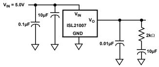
FIGURE 55. HANDLING HIGH LOAD CAPACITANCE
