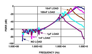
FIGURE 8. PSRR vs CAPACITIVE LOADS
