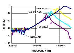
FIGURE 21. PSRR vs CAPACITIVE LOADS
