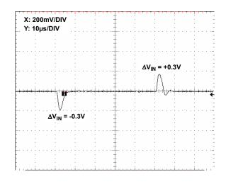
FIGURE 36. LINE TRANSIENT RESPONSE, NO CAPACITIVE LOAD
