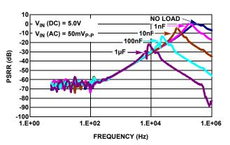
FIGURE 48. PSRR vs CAPACITIVE LOADS
