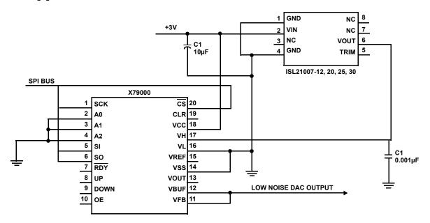
FIGURE 1. TYPICAL APPLICATION PRECISION 12-BIT SUBRANGING DAC
