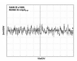
FIGURE 13.  $V_{OUT}$  NOISE, 0.1Hz TO 10Hz
