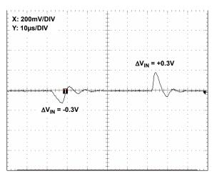
FIGURE 10. LINE TRANSIENT RESPONSE, 0.001µF LOAD **CAPACITANCE**
