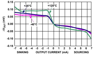
FIGURE 6. LOAD REGULATION OVER TEMPERATURE
