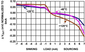
FIGURE 46. LOAD REGULATION OVER TEMPERATURE
