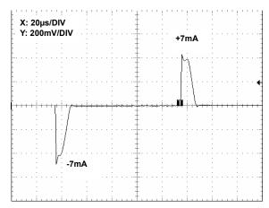
FIGURE 28. LOAD TRANSIENT RESPONSE, NO CAPACITIVE LOAD
