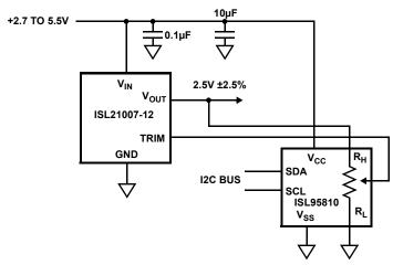
FIGURE 59. OUTPUT ADJUSTMENT USING THE TRIM PIN
