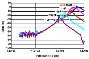
FIGURE 35. PSRR vs CAPACITIVE LOADS
