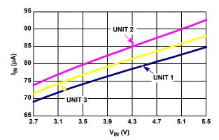
FIGURE 15.  $I_{IN}$  vs  $V_{IN}$  (3 UNITS)
