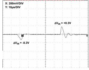
FIGURE 37. LINE TRANSIENT RESPONSE, 0.001µF LOAD CAPACITANCE
