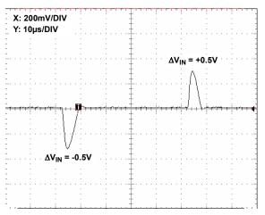
FIGURE 49. LINE TRANSIENT RESPONSE, NO CAPACITIVE LOAD
