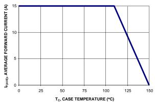
Figure 1: Current Derating Curve, Per Element
