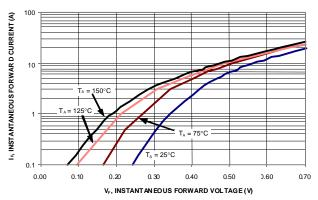
Figure 2: Typical Forward Characteristics, Per Element
