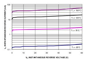
Figure 3: Typical Reverse Characteristics, Per Element
