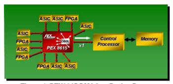
Figure 4. PEX8615 DMA in a Packet Router
