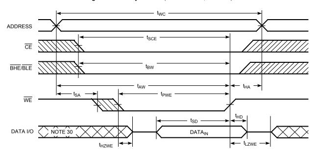
Figure 9. Write Cycle No. 4  $(\overline{BHE/BLE}\ Controlled,\ \overline{OE}\ LOW)^{[28,\ 29]}$
