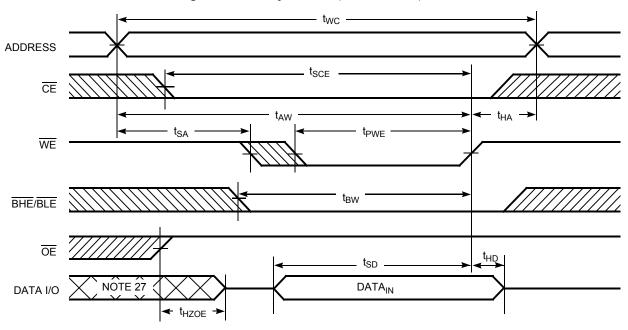
Figure 7. Write Cycle No. 2  $(\overline{\text{CE}} \text{ Controlled})^{[23, 24, 25, 26]}$
