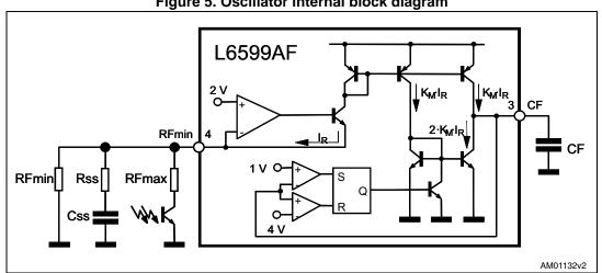
Figure 5. Oscillator internal block diagram
