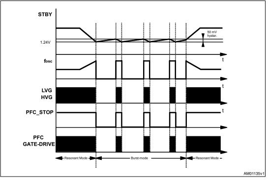
Figure 8. Load-dependent operating modes: timing diagram
