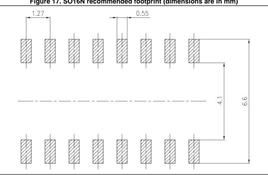
Figure 17. SO16N recommended footprint (dimensions are in mm)
