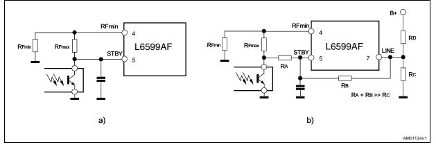
Essentially,  $RF_{max}$  defines the switching frequency  $f_{max}$  above which the L6599AF enters burst mode operation. Once  $f_{max}$  is fixed,  $RF_{max}$  is found from the relationship:
