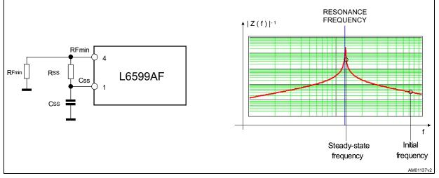
As a result, the average input current smoothly increases, without the peaking that occurs with linear frequency sweep, and the output voltage reaches the regulated value with almost no overshoot.
