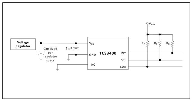
$V_{BUS}$  in the above figures refers to the I<sup>2</sup>C bus voltage which is either  $V_{DD}$  or 1.8V. Be sure to apply the specified I<sup>2</sup>C bus voltage shown in the Ordering & Contact Information for the specific device being used.
