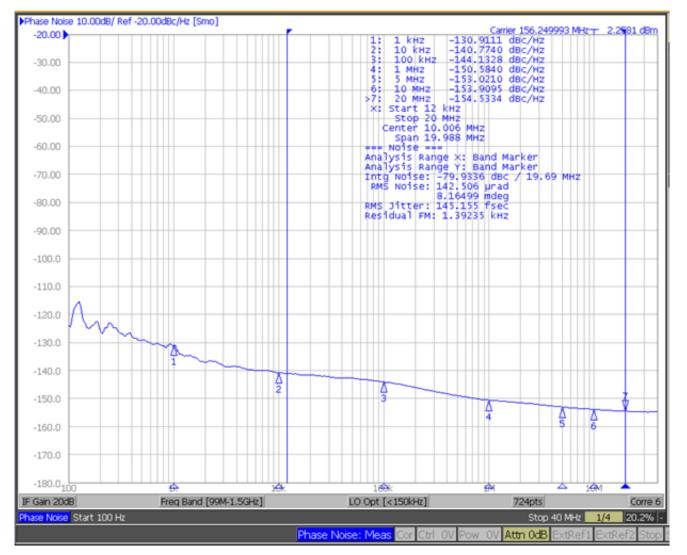
Phase jitter = 145fs<sub>rms</sub>, 156.25MHz carrier frequency; integration range: 12kHz–20MHz
