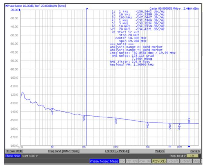
Phase jitter = 204fs<sub>rms</sub>, 100MHz carrier frequency; integration range: 12kHz-20MHz
