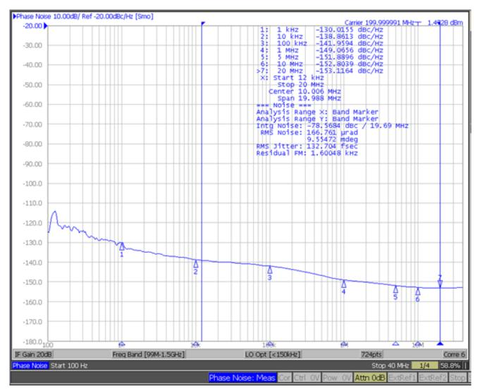
Phase jitter = 132fs<sub>rms</sub>, 200MHz carrier frequency; integration range: 12kHz–20MHz
