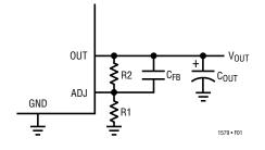
Figure 1. Adjustable Operation
