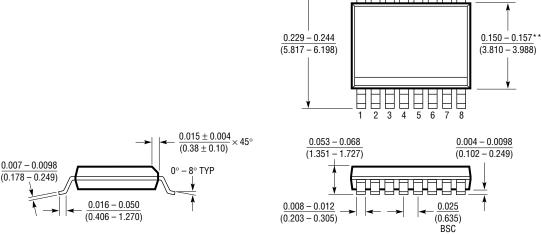
\* DIMENSION DOES NOT INCLUDE MOLD FLASH. MOLD FLASH SHALL NOT EXCEED 0.006" (0.152mm) PER SIDE
