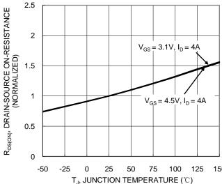
Figure 6. On-Resistance Variation with Junction Temperature
