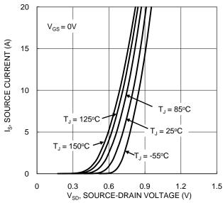
Figure 9. Diode Forward Voltage vs. Current
