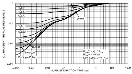
Figure 12. Transient Thermal Resistance
