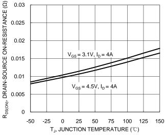
Figure 7. On-Resistance Variation with Junction Temperature
