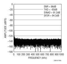
Figure 6b. 32k Point FFT Plot with f<sub>IN</sub> = 2kHz for Circuit Shown in Figure 6a
