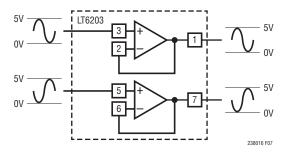
Figure 7. LT6203 Buffering a Fully Differential Signal Source
