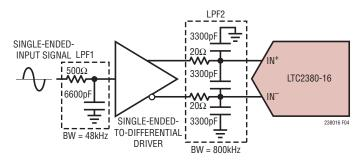
Figure 4. Input Signal Chain
