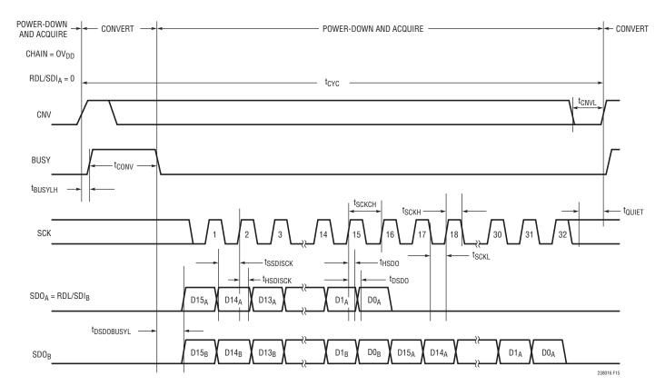
Figure 15. Chain Mode Timing Diagram
