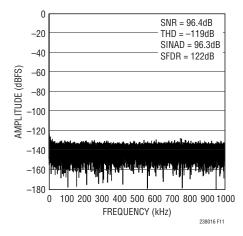
Figure 11. 32k Point FFT with  $f_{IN}$  = 2kHz of the LTC2380-16
