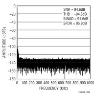
Figure 9b. 32k Point FFT Plot with f<sub>IN</sub> = 2kHz for Circuit Shown in Figure 9a
