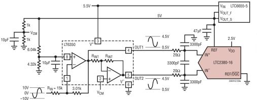
Figure 9a. LT6350 Configured to Accept a ±10V Input Signal While Running Off of a Single 5.5V Supply When Digital Gain Compression Is Enabled in the LTC2380-16
