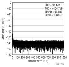
Figure 5b. 32k Point FFT Plot with  $f_{\text{IN}}$  = 2kHz for Circuit Shown in Figure 5a
