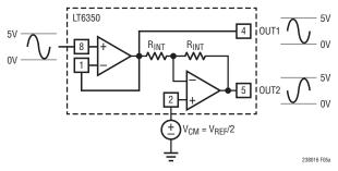
Figure 5a. LT6350 Converting a OV-5V Single-Ended Signal to a ±5V Differential Input Signal
