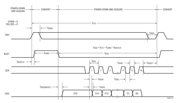
Figure 13. Using a Single LTC2380-16 in Normal Mode
