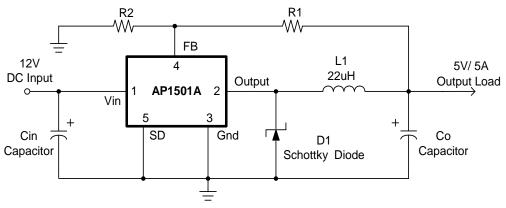
$$V_{OUT} = V_{FB} \times (1 + \frac{R1}{R2})$$
