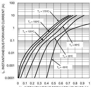
V<sub>F</sub>, INSTANTANEOUS FORWARD VOLTAGE (V) Figure 2 Typical Forward Characteristics
