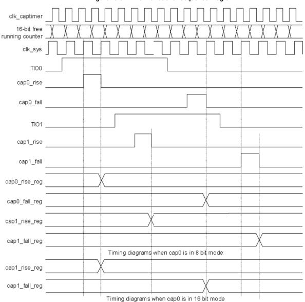
Figure 19-3. Timer Functional Sequence Diagram
