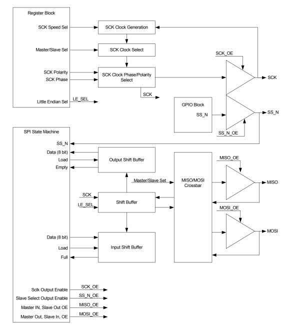
Figure 18-1. SPI Block Diagram
