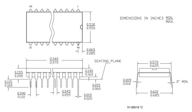
Figure 24-3. 40-Pin (600-Mil) Molded DIP P17
