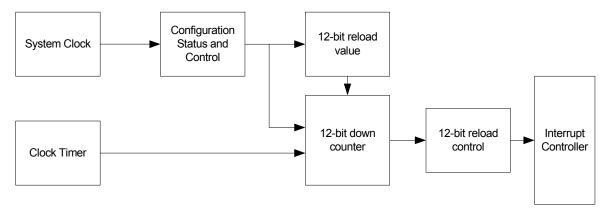
Figure 13-2. Programmable Interval Timer Block Diagram
